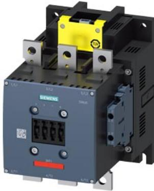
Power contactor, AC-3 225 A, 110 kW / 400 V Coil AC 50/60 Hz and DC 200-277 V x (0.8-1.1) F-SPS input 24 V DC 3-pole size S10 Auxiliary contacts 2 NO + 2 NC permanently mounted Main circuit: Busbar Control and auxiliary circuit: Screw terminal
