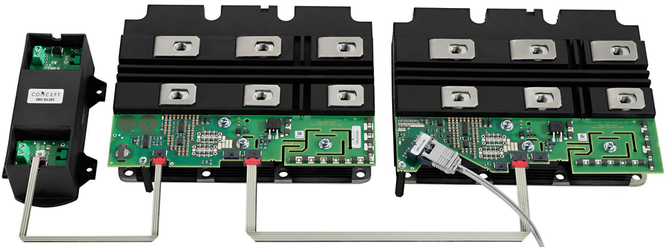
Fig. 1 1SP0335D (slave) with 1SP0335V (master) each screwed onto a 6.5kV IGBT module (left: DC/DC converter ISO5125I connected to 1SP0335D)
