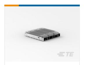
TE Part #4-2170740-1 QSFP28, 1X3, CAGE ASSY, SPRING, HS, LP
