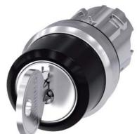
RONIS key-operated switch, 22 mm, round, metal, shiny, lock number SB30, with 2 keys, 3 switch positions I-O-II, latching, actuating angle  $2x45^{\circ}$ , 10:30h/12h/13:30h, Key removal I+O+II, possible special locks: SB31, 421, 455
