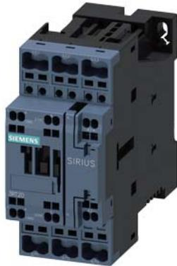
power contactor, AC-3e/AC-3, 25 A, 11 kW / 400 V, 3-pole, 48 V DC, auxiliary contacts: 1 NO + 1 NC, spring-loaded terminal, size: S0
