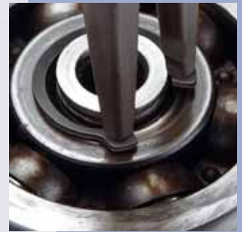
Heavy duty tips: optimum stability when loosening tight circlips
