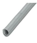
Protective hose, material: PVC, filament: PVC sheathed spring steel, UV-resistant: no, flexible, degree of protection: IP68, color: gray, inner diameter: 22 mm, Total length: 10 m
