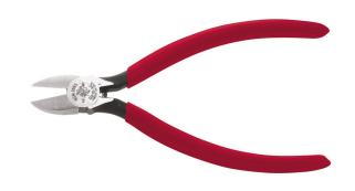
These Klein Tools Diagonal Cutting Pliers are designed with spring-loaded jaws for a self opening action. Their shortened jaws and beveled cutting edges permit close cutting in tight spaces. The induction hardened cutting knives made of US-forged steel, allow for a long lasting knife life.
