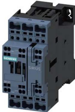
Traction contactor, AC-3 25 A, 11 kW / 400 V 1 NO + 1 NC with electronic drive 72 V DC, 0.7-1.25\* US, with integrated varistor, 3-pole, Size S0, Spring-type terminal
