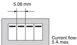
More than two relays can be closely mounted upside down as shown in the following illustration.
