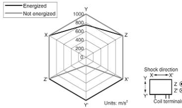
Measurement conditions: Impose a shock in the ±X, ±Y, and ±Z directions three times each with the Relay energized to check the shock values that cause the Relay to malfunction.
