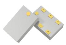
The DC2337J5020AHF is a low cost, low profile sub-miniature high performance 20 dB directional coupler in an easy to use Xinger style surface mount package. It is designed for 2300 – 3700MHz applications including: 5G, LTE and ISM. The DC2337J5020AHF is ideal for power detection, signal injection and other applications where low insertion loss signal monitoring is required. The DC2337J5020AHF is available on tape and reel for pick and place high volume manufacturing.
