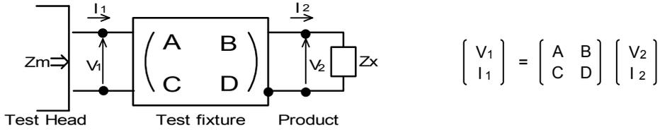
(2) The impedance of chip coil  $Z_x$  and measured value  $Z_m$  can be described by input/output current/voltage.
