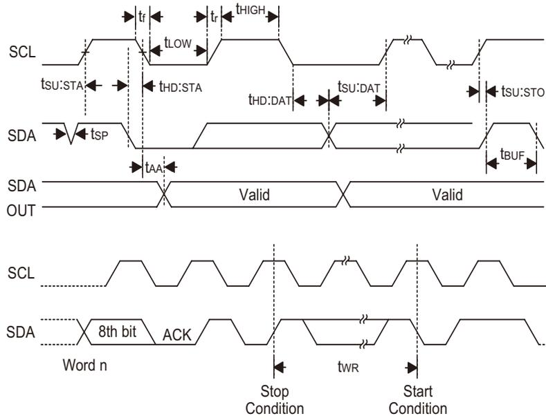
Note: The write cycle time  $t_{WR}$  is the time from a valid stop condition of a write sequence to the end of the valid start condition of sequential command.
