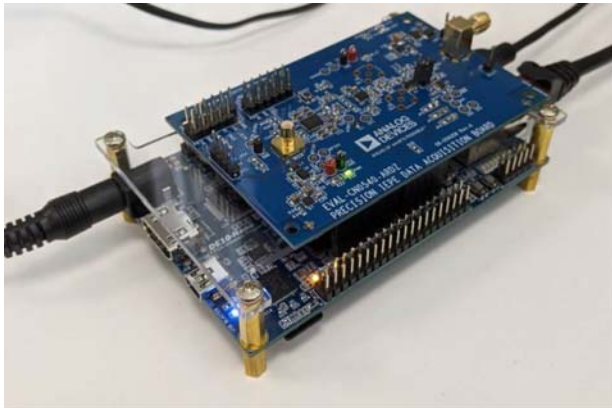
Figure 18. EVAL-CN0540-ARDZ Mounted on Terasic DE10-Nano Carrier Board
