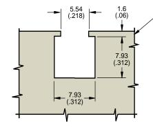
NOTE: When attachment is made, this edge of sheet and under surface of attached material must be in contact with each other.
