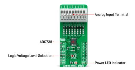
Each bit of the 8-bit serial word corresponds to one switch of the device. Internal switching channels are independently controlled by an individual bit, providing an option of having any, all, or none of the switches activated. All of the input channels of the multiplexer can be easily connected to a nine pole spring action block terminal, without having to use any additional tools, such as screwdrivers, while the output pin from the multiplexer is routed to the AN pin on the mikroBUS™ socket.
