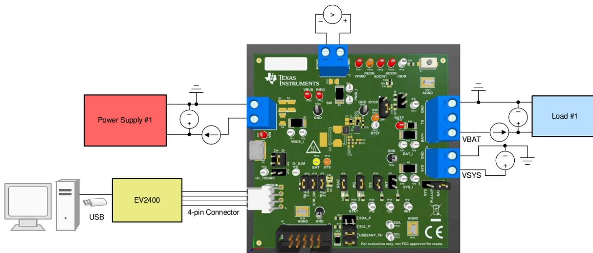
**Figure 2-1. Test Setup for BQ25638x EVM**
