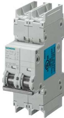
Miniature circuit breaker 240 V 14kA, 2-pole, C, 25A, D=70 mm according to UL 489
