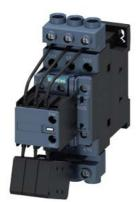
Capacitor contactor, AC-6b 33 kVAr, / 400 V 1 NO + 2 NC, 110 V AC, 50 Hz 3-pole, Size S0 screw terminal
