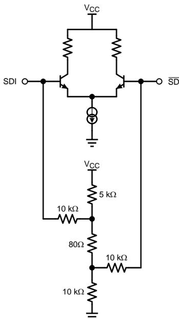
Figure 3. Differential Input Stage for SDI and  $\overline{\text{SDI}}$ .
