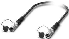
M17 MPO series with preassembled FO plug assembly: 24-pos. plug-plug, multimode fiberglass G62.5/125  $\mu\text{m}$  OM1, with screw connection, length of FO cable: 30 m, IP67 degree of protection after being inserted, fixed installation in cable ducts, underground cable ducts, and cable protection pipes for indoor/outdoor use
