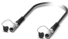
M17 MPO series with preassembled FO plug assembly: 24-pos. plug-plug, multimode fiberglass G62.5/125  $\mu\text{m}$  OM1, with screw connection, length of FO cable: 10 m, IP67 degree of protection after being inserted, fixed installation in cable ducts, underground cable ducts, and cable protection pipes for indoor/outdoor use
