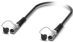
M17 MPO series with preassembled FO plug assembly: 24-pos. plug-plug, multimode fiberglass G62.5/125  $\mu\text{m}$  OM1, with screw connection, length of FO cable: 120 m, IP67 degree of protection after being inserted, fixed installation in cable ducts, underground cable ducts, and cable protection pipes for indoor/outdoor use
