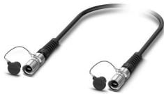
M17 MPO series with preassembled FO plug assembly: 24-pos. plug-plug, multimode fiberglass G62.5/125  $\mu\text{m}$  OM1, with screw connection, length of FO cable: 190 m, IP67 degree of protection after being inserted, fixed installation in cable ducts, underground cable ducts, and cable protection pipes for indoor/outdoor use
