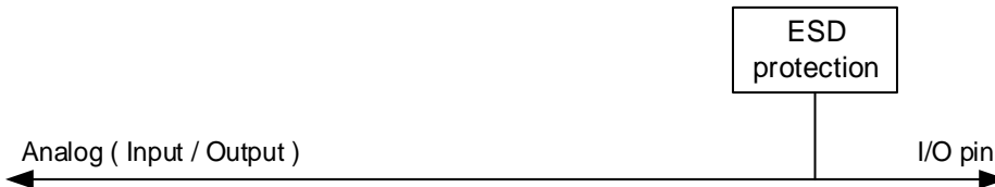
Figure 7-4. Basic structure of Analog configuration
