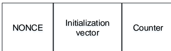
Figure 23-12. Counter block structure
