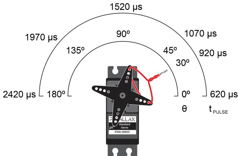
The relationship between angle ( $\theta$ ) and  $t_{PULSE}$  follows these two equations. The first is for determining  $t_{PULSE}$  for a desired angle ( $\theta$ ), and the second is the inverse, for determining angle ( $\theta$ ) given a certain  $t_{PULSE}$ .
