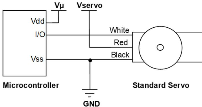
\* V $\mu$  and Vservo are typically different supplies. This prevents sudden increases in servo current under load from causing a brown-out condition in the microcontroller. Some designs do use a single regulator to supply both, but only when the microcontroller allows a supply in the 4-6 V range and the voltage regulator supplying both devices can hold its output voltage while supplying enough current to all connected servos at simultaneous peak current.
