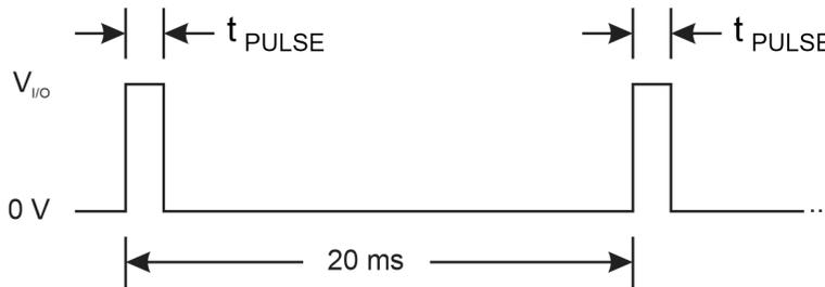
Here are some examples of  $t_{PULSE}$  durations for common angular positions ( $\theta$ ). This setup assumes that the servo horn was unscrewed and removed from the spline, then pressed back on with the jumper wire pointing at  $0^\circ$  while the microcontroller was sending the servo  $t_{PULSE} = 620 \mu$ s signals. After that, the other  $t_{PULSE}$  signals will result (approximately) in the other corresponding angles.
