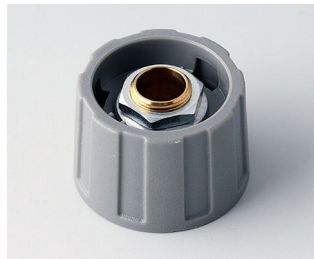
A2523638 ROUND KNOB 23, without line ABS (UL 94 HB) dusty gray RAL 7037 23x15mm 1/4"
