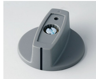
A2440068 SPINDLE-SHAPED KNOB 40, with line ABS (UL 94 HB) dusty gray RAL 7037 40x16mm 6mm
