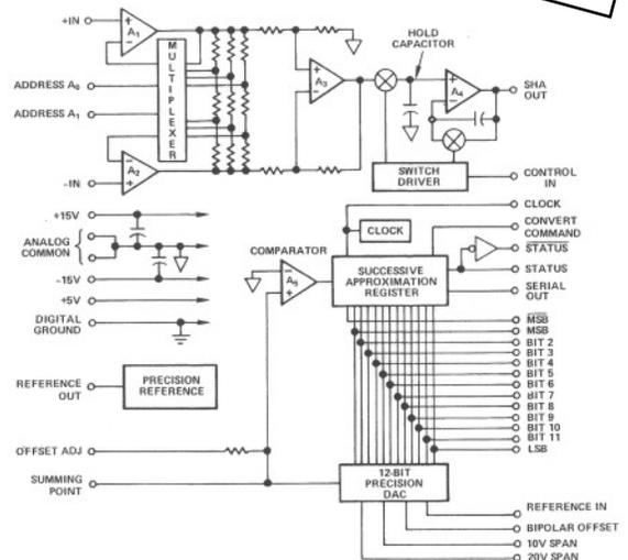
Figure 1. DAS1151 Block Diagram and Pin Designations
