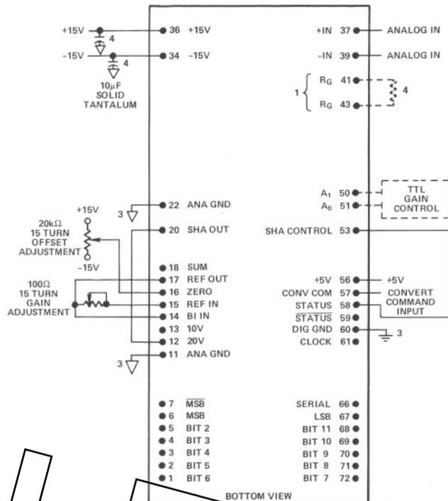
Figure 3. Module Connections for  $\pm 10V$  Range
