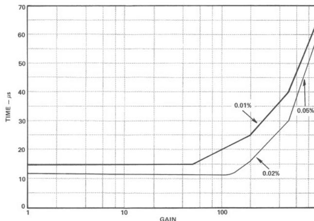
Figure 4. Typical Settling Time Curves for DAS1150
