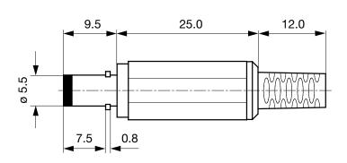
Cable diameter max. 4.0 mm
