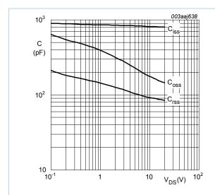
Fig. 16. Input, output and reverse transfer capacitances | Fig. 17. Source (diode forward) current as a function of as a function of drain-source voltage; typical values
