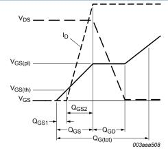
Fig. 14. Gate charge waveform definitions
