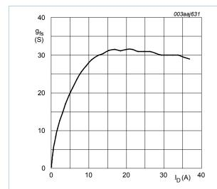
Fig. 6. Forward transconductance as a function of drain current; typical values
