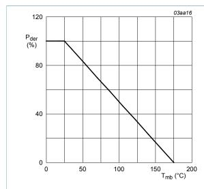
Normalized total power dissipation as a Fig. 1. function of mounting base temperature
