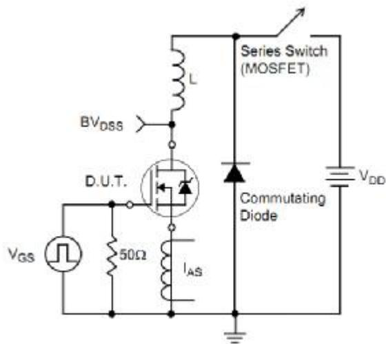
Figure 7. Unclamped Inductive Switching Test Circuit
