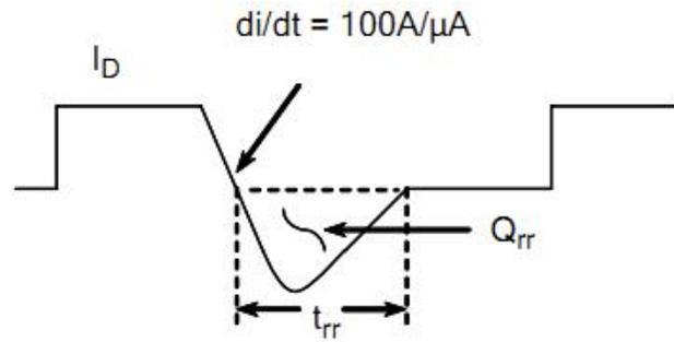
Figure 6. Diode Reverse Recovery Waveform
