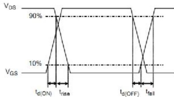
Figure 4. Resistive Switching Waveforms
