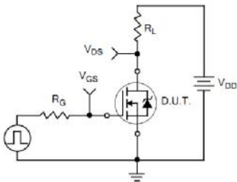
Figure 3. Resistive Switching Test Circuit
