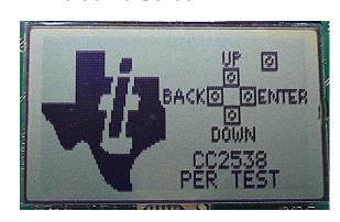
Turn on power with the Main Power switch. You should now see the Texas Instruments logo and a short description of the buttons on the LCD. Pushing any of the five buttons on the board will take you to the main menu.
