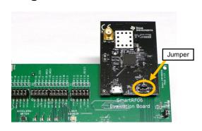
Insert a CC2538-CC2592EM board into the SmartRF06EB as shown above.
