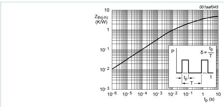
Fig. 3. Transient thermal impedance from junction to heatsink as a function of pulse width
