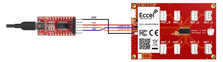
Figure 3-3. Pepper C1 FCC MUX - schematic connection with the USB-UART converter
