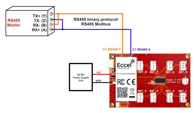
Figure 3-6. Pepper C1 FCC MUX RS485 - half duplex connection schematic
