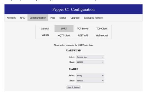
Figure 3-2. Console logs on the UARTO/USB
