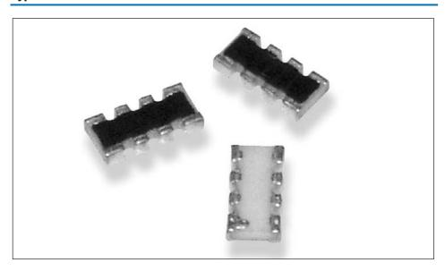
The MRS series is an entirely new chip network utilising nickel chrome sputtering on high purity alumina. This network has been designed for high volume applications and is offered with 4 isolated resistors on a single substrate (4 x 0603 resistors) at 0.1% with convex terminals. A wide value range and alternative TCRs (Temperature Coefficient of Resistance) make this a most versatile resistor solution.
