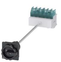
SENTRON, Switch disconnector 3LD, main switch, 6-pole, lu: 25 A, Operating power / at AC-23 A at 400 V: 9.5 kW, floor mounting with door coupling, rotary operating mechanism, black, 4-hole mounting of the handle
