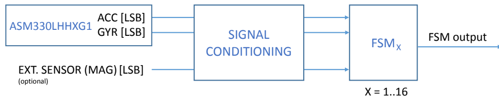
Figure 2. State machine in the ASM330LHHXG1
