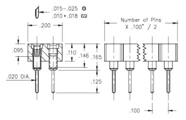
**Description:** Interconnect Socket Standard Solder Tail Socket Accepts .015"- .025" (0,38 - 0,635 mm) dia leads Double Row Through Hole Plating Code: Shell Plating:
