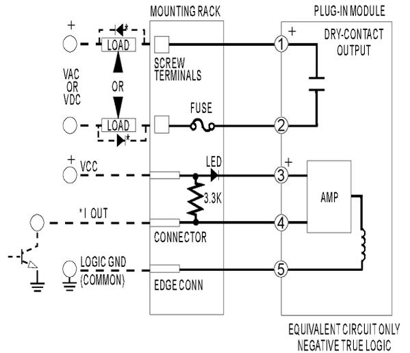
\* Commutating diode\* must be used on inductive loads (Typical: 1N4005).
