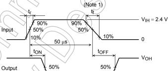
Note 1: Pulse Width 50 μs, Duty Cycle 10% Output Impedance 50  $\Omega$ ,  $t_f \le 5$  ns,  $t_f \le 10$  ns
