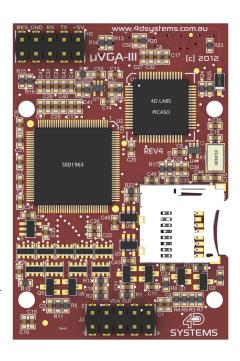
This module serves as a perfect solution to connect to an external VGA monitor for an application requiring animation, slideshows, images or sound. This **PICASO**-driven Intelligent Display Module is a perfect example of where art meets technology.
