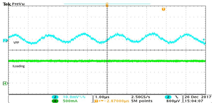
Figure 5. TPS65295EVM-079 VPP Ripple,  $I_{OUT} = 1$  A
