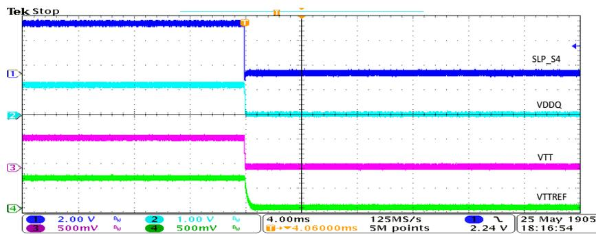
Figure 7. TPS65295EVM-079 Power Down Relative to SLP\_S4
