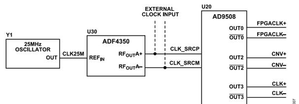
Figure 7. Simplified Diagram of the Clock Circuitry
