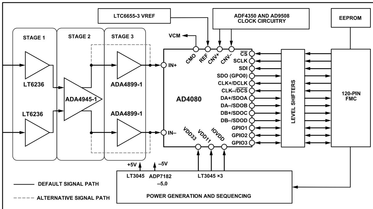
Figure 2. Simplified Block Diagram of the EVAL-AD4080-FMCZ
