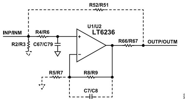
Figure 3. Stage 1 Simplified Schematic
