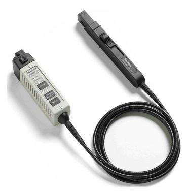
TCP0030A is a high-performance, easy-to-use AC/DC current probe designed for use and direct connection to oscilloscopes with the TekVPI™ probe interface. This AC/DC current measurement probe provides greater than 120 MHz of bandwidth with selectable 5 A and 30 A measurement ranges. It also provides exceptional low-current measurement capability and accuracy to current levels as low as 1 mA, important for meeting today's challenging current measurement needs.
