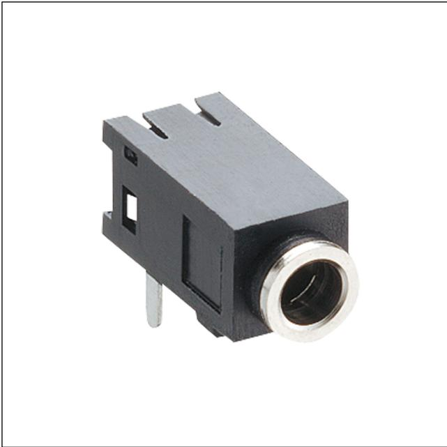
Jack chassis socket acc. to JIS C 6560 JC25J3A, 2.5 mm, 3 poles/stereo, angular version, with metal collar, for printed circuit boards
